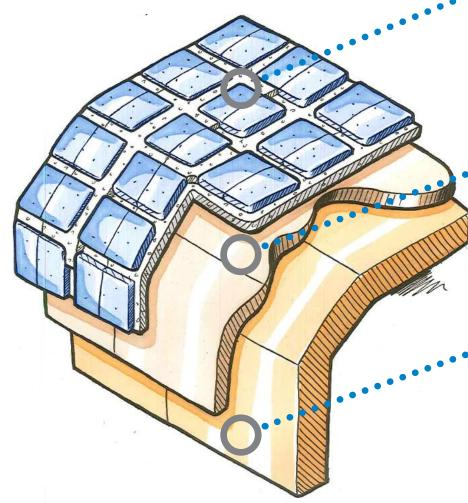
It is the composite structure of the 3 materials working together which provides the unique properties of the absolute-pools Pre-formed pool shell.
